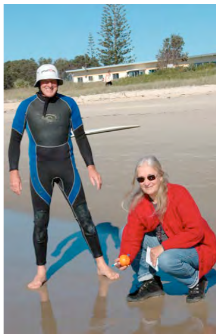
Collecting an orange. Citizens studied local near-shore sea currents by releasing tagged oranges. When collected, these revealed the likely trajectory of effluent.
